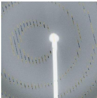
**Figure 10. The XDS findings are visualized using MOSFLM by converting the orientation matrix from XDS into MOSFLM format. This conversion also includes the distance, beam center, and mosaicist. The generated descriptions may be easily imported into MOSFLM, which provides interactive capabilities for displaying forecasts, analyzing the beam center or ice rings, and modifying mosaicist settings.**
